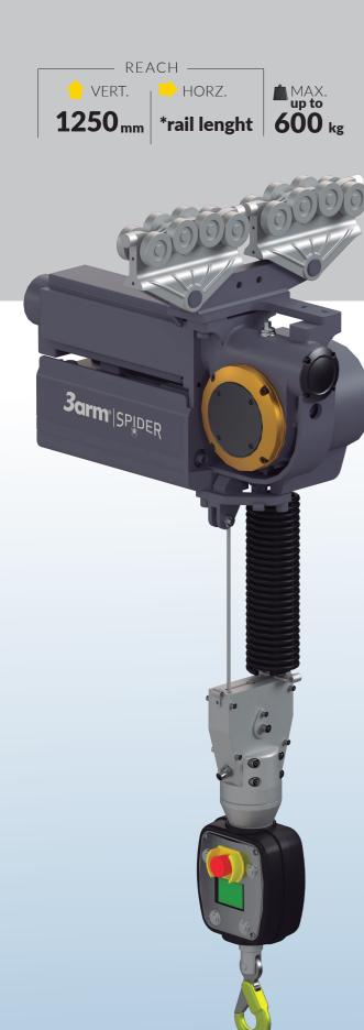
The 3arm Smart Lift Spider 600R is an electronic rope balancer designed to be mounted on rail systems for manually handling loads up to 600kg
