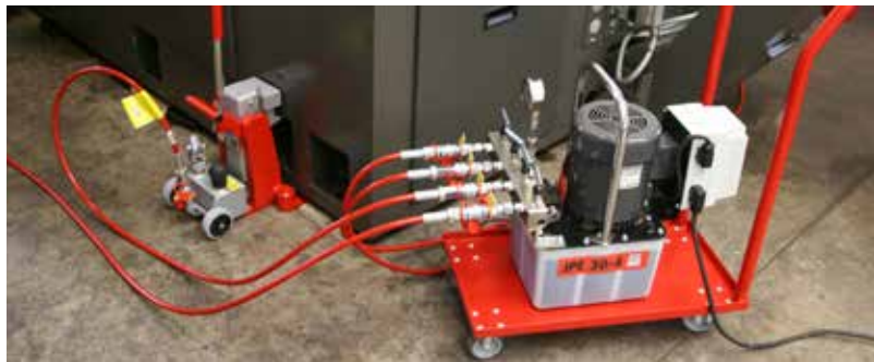
Electric pump JPE 30/4 NVR with 4 jacks in operation.
