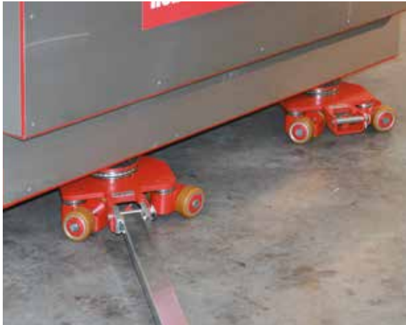
Example as tandem transport trolley
