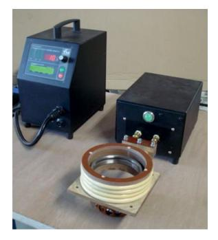
TM has also developed a smaller version, mid frequency, for ball bearings max. ø 100 mm. It is operated entirely manually.
